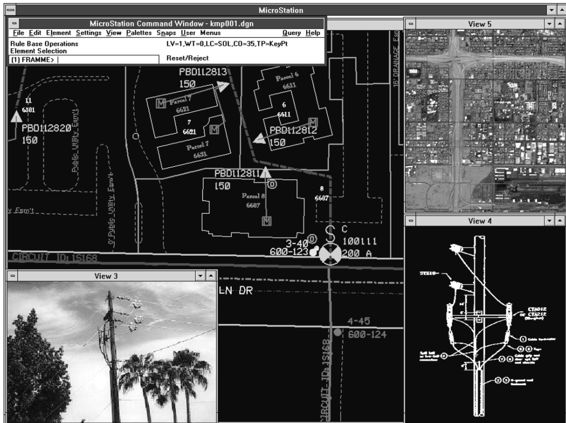
Electric utility data in a GIS.
